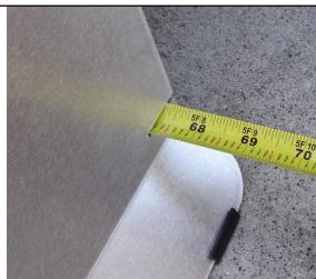
The rear tape measurement (side towards the rear of the vehicle) minus the front tape measurement (side closest to the front of the vehicle) is the total toe of the axle. A larger measurement on the front side indicates toe out, and a larger measurement on the rear side indicates toe in.
