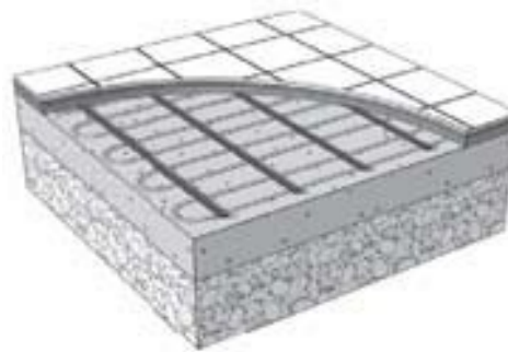
MA ICE-30 cable under tile
