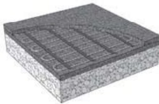
MA ICE-30 cable in asphalt
