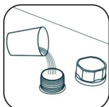
②.ÖPPNA VATTENUTSLUTET FÖR ATT TILLFÖRA KYLVATTEN (SPILLA INTE UT VATTEN!).
