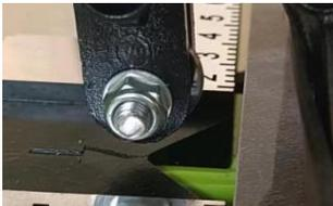
The first tool wheel is stuck in the machine head tool rest. Use M6\*25 screws to Pierce the hole from the outside and tighten the nut.
