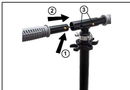
Press button (1), then slide the handle (2) until button (1) fits into slot (3).
