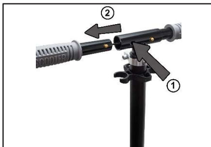
To fold the handle, press button (1) located in slot (3) and pull out the handle (2).
