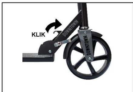
3. While holding the release lever up, push the steering column forward till you hear a „click“.
