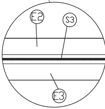
S3 must be stuck on the top gap of E2 & E3
