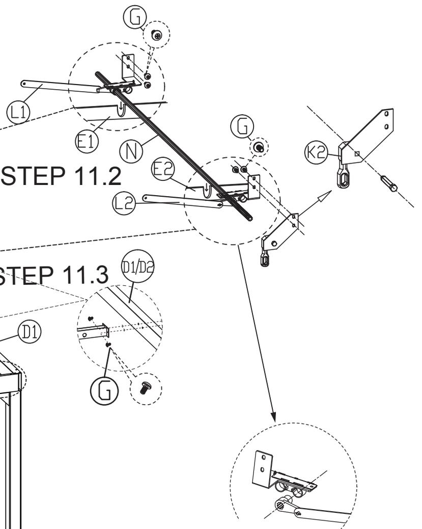
If L1/L2 breaks into two parts, it need to be reassembled.
