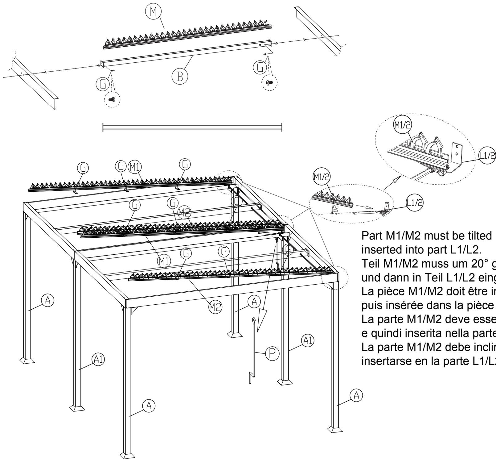
Part M1/M2 must be tilted 20° and then inserted into part L1/L2.
