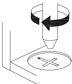
**EN**\_Turn cam lock clockwise to tighten.
