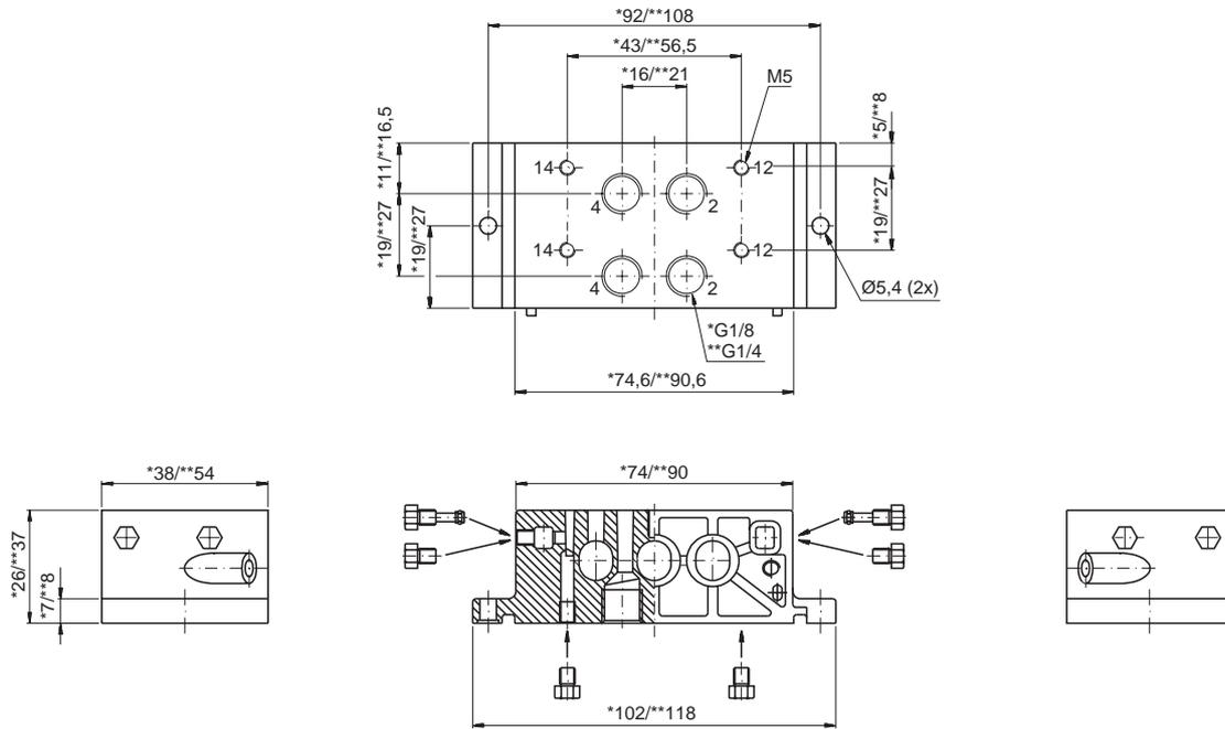
**Intermediate manifold 18 to 26 mm**
