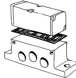
A specially designed seal between the valve and manifold, with a positive seal around the outer edge, prevents dirt from finding its way into the gap between the valve and manifold. The fully 'convex' contour guarantees a perfectly clean joint, with no possibility of dirt or bacteria build-up.
