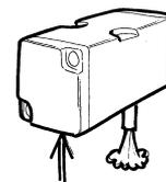
Flow rates through P2V-B valves are about 10% higher than for the majority of ISO 1 valves (P2V-B C = 4.4 NI/s, bar). Flows through the valve itself are so high that it is the standardised hole connection pattern that prevents higher flow rates being achieved.
