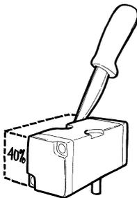
The width of the manifold of P2V-A valves is about 60% less than that of normal ISO1 valves, while that of the P2V-B valves is about 40% less, which means that more valves can be accommodated in the same space.
