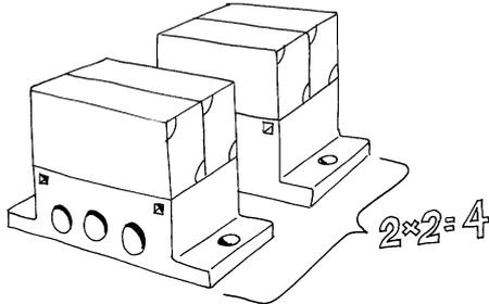
Each multiple manifold is designed with two valve positions to save time and cost when mounting. Only two manifolds are required, for example, to mount four valves, as against four traditional manifolds. This halves the mounting time, while reducing the risk of leakage between manifolds as a result of fewer joints.
