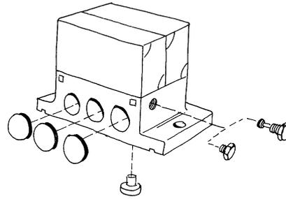
The same multiple manifold can be used for all variants of P2V-A/B valves, whether pneumatically operated or electrically operated and with internal or separate air supply to the pilot valves.
