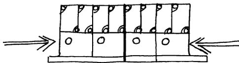
Several variants of connecting blocks are available, allowing connection from the top, bottom or side. Plugs can be fitted to interrupt connections between multiple manifolds, allowing (for example) the two sides of the manifold to be supplied at different pressures.
