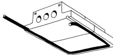
The underside of the multiple manifolds contains a groove for an O-ring-type seal, enabling it to be fitted inside a valve cubicle so that only a single rectangular opening is required for all connections through the cubicle wall, while the seal maintains integrity of the cubicle enclosure in respect of external dust and moisture.
