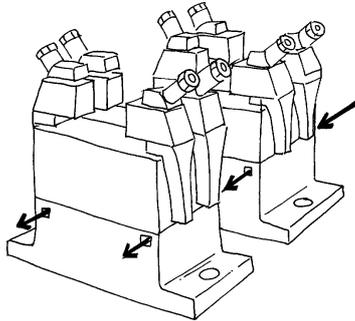
Multiple manifolds have common through channels for separate supply of compressed air to the pilot valves and exhaust from them. Connections can be made to these channels at any connection block. The pilot valves can also be supplied and/or vented individually.
