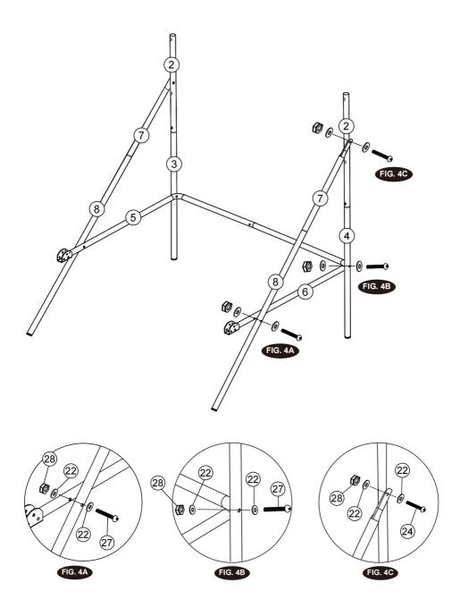
8. Attach the Short Horizontal Cross Brace (#12) to the Vertical Board Support Mounting Tubes (#2) using Bolts
