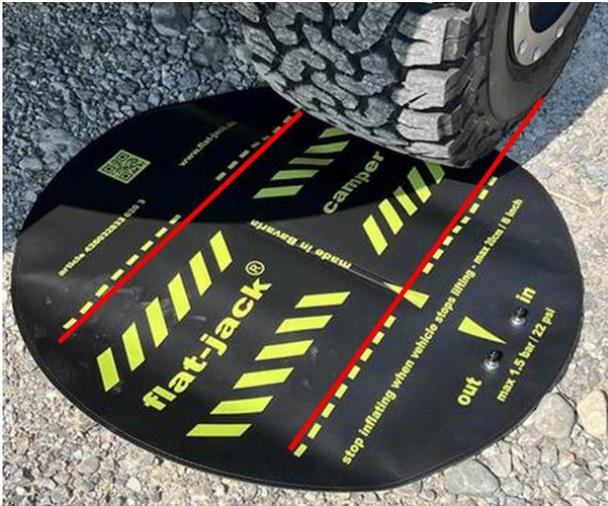
Image 6: Correct positioning of the flat-jack®
