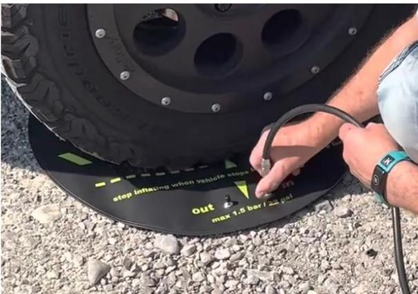
Image 11: Connecting the air pump
