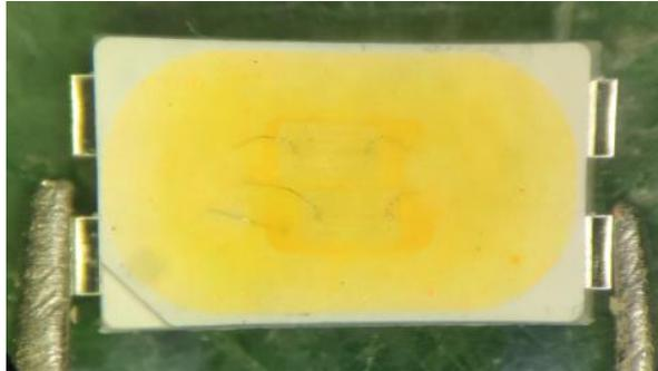
(3) When populating boards in SMT production, there are basically no restrictions regarding the form of the pick and place nozzle, except that mechanical pressure on the surface of the resin must be prevented. This is assured by choosing a pick and place nozzle which is larger than the LED's reflector area.
