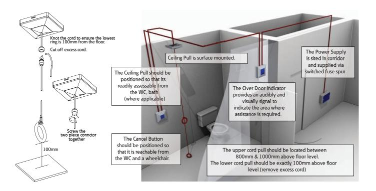
All system components are designed to be sited internally and positioned in locations where they are readily accessible by the user. The area should be clean and dry and sound and light levels allow the status of all device indicators and sounders to be seen and heard.
