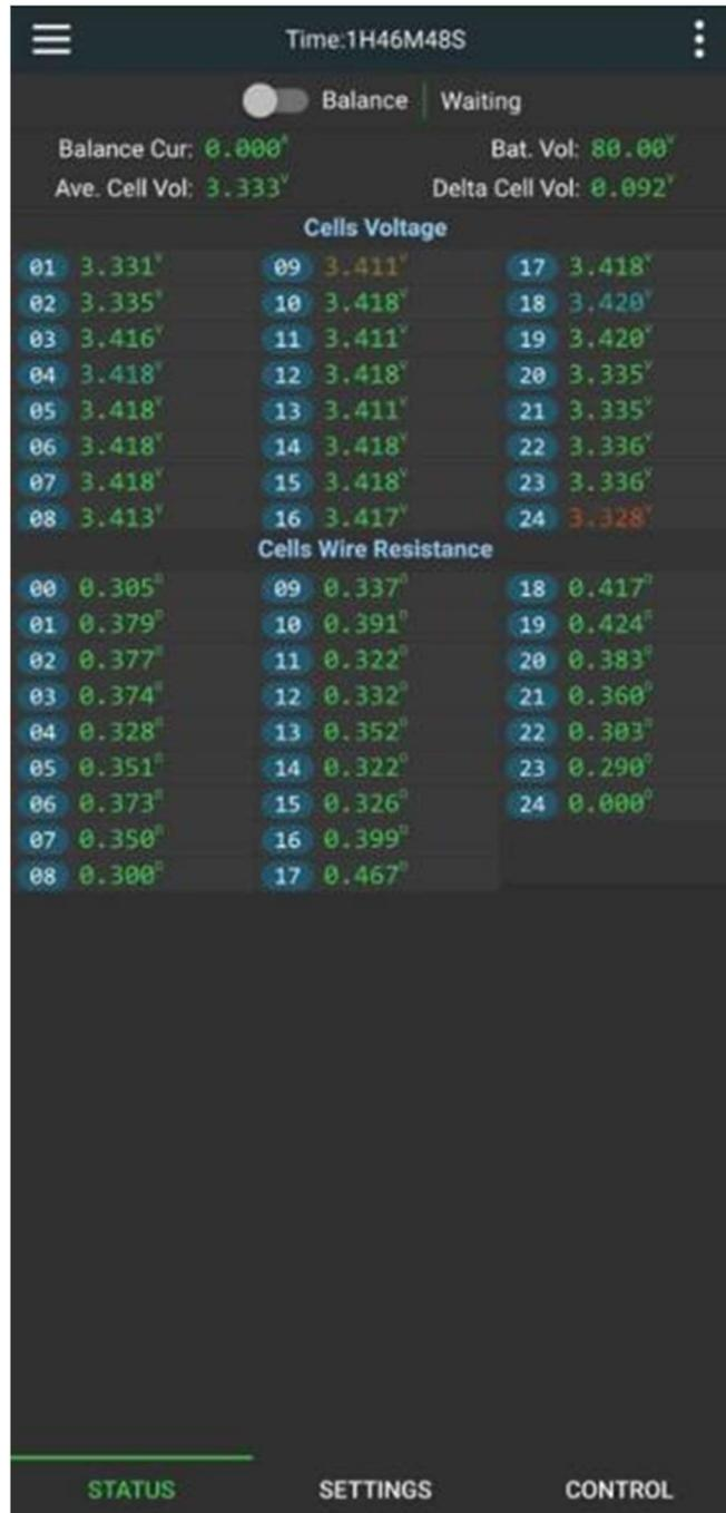
On the Real-Time Status page, you can view information such as switch status, charging current, discharge current, temperature display, protection alarm, individual voltage, total battery voltage, maximum pressure difference, average single voltage, balanced status, balanced current, balanced line resistance, etc.
