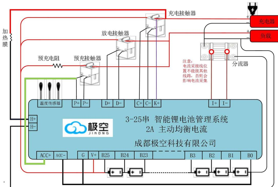
Wiring mode of serial battery pack system
