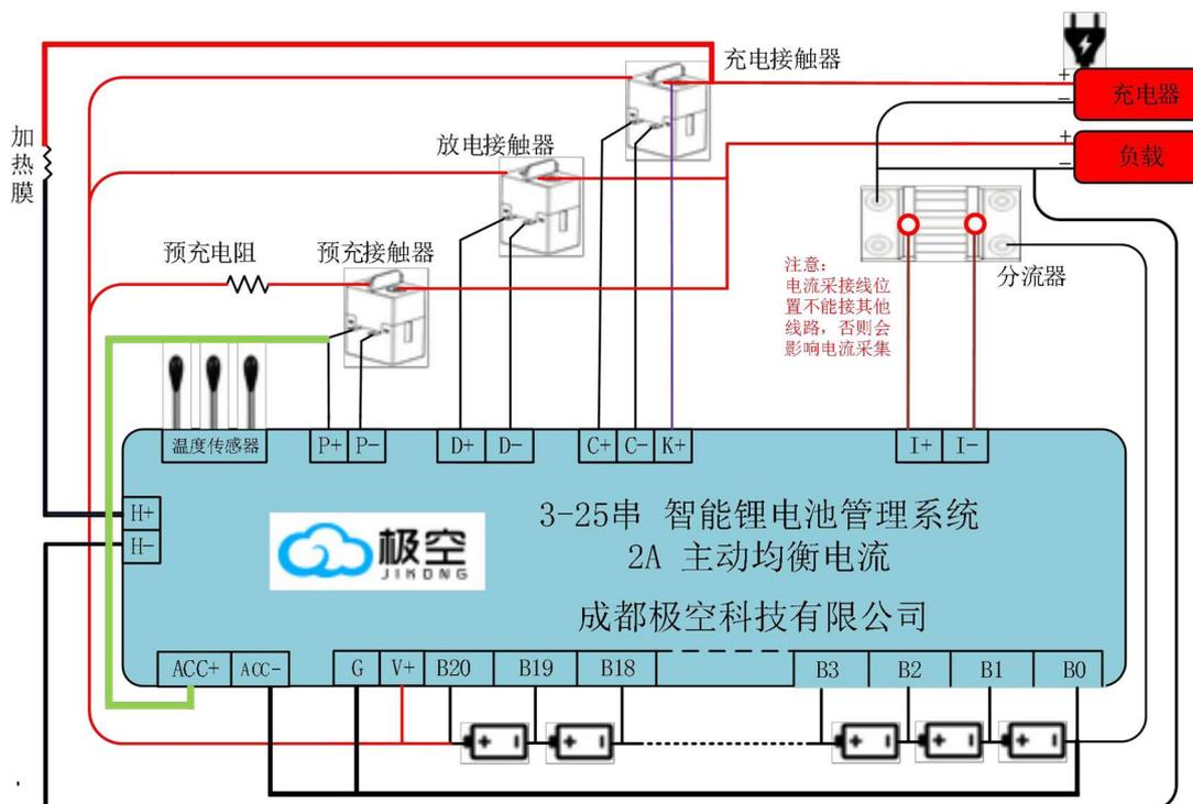
The 20 Strial battery wiring diagram is shown.
