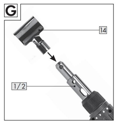
The hot air deflector can be used with the hot air attachment. This is helpful e.g. when shrinking cables.
