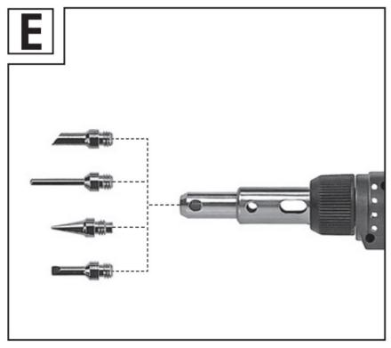
The gas soldering iron is provided with the blow torch attachment, hot air/soldering attachment and with a soldering tip can be used as soldering iron.
