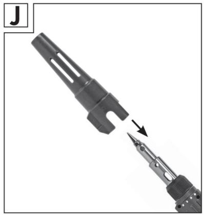
The contents include a protective cap (15). Use the protective cap to safely rest the hot device and to prevent mechanical hazards.
