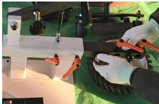
3. Insert the circular grinder into the tool arm and lock the handle
