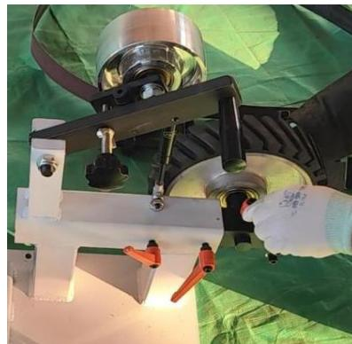
4. After hanging the sand belt, press down on the black handle to pull the tool arm out as much as possible, then lock the handle and gently lift the black handle to tension the sand belt.
