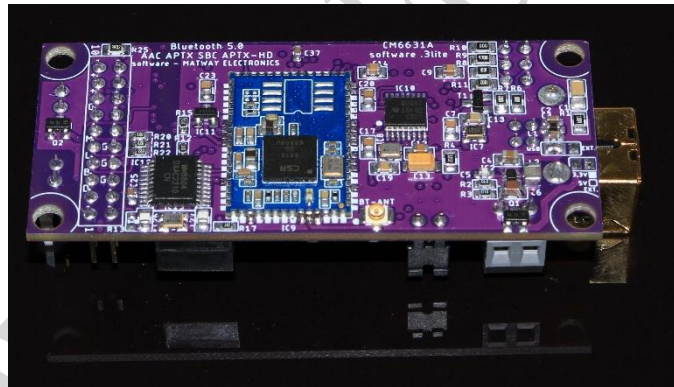
Photo. 3 PCB Preview – BOTTOM (USB+BT / I2S + SPDIF version)
