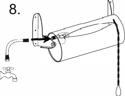
After connecting the water supply or storage tank and turning on the water supply, the body of the dumping device will begin to fill with water automatically.
