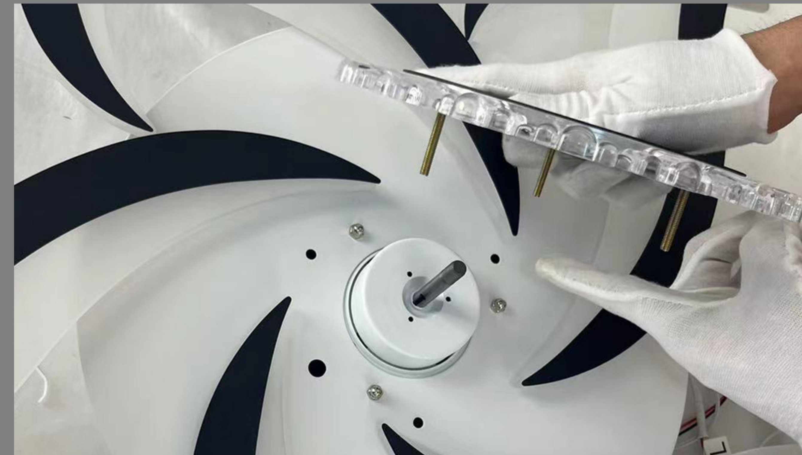
Step 5: Apply acrylic and align it with the hole position
