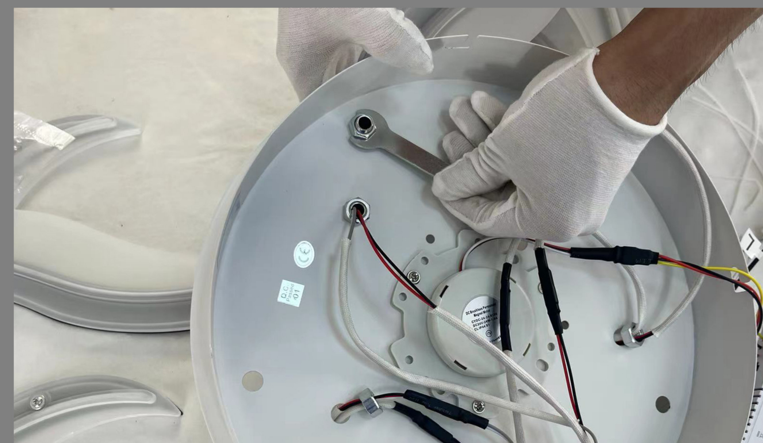
Step 3: Use a wrench to secure the nut
