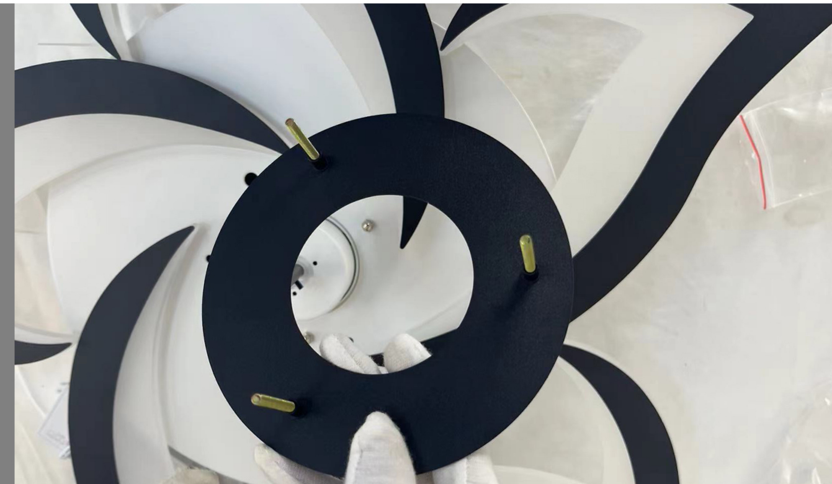
Step 4: Fix the film with screws
