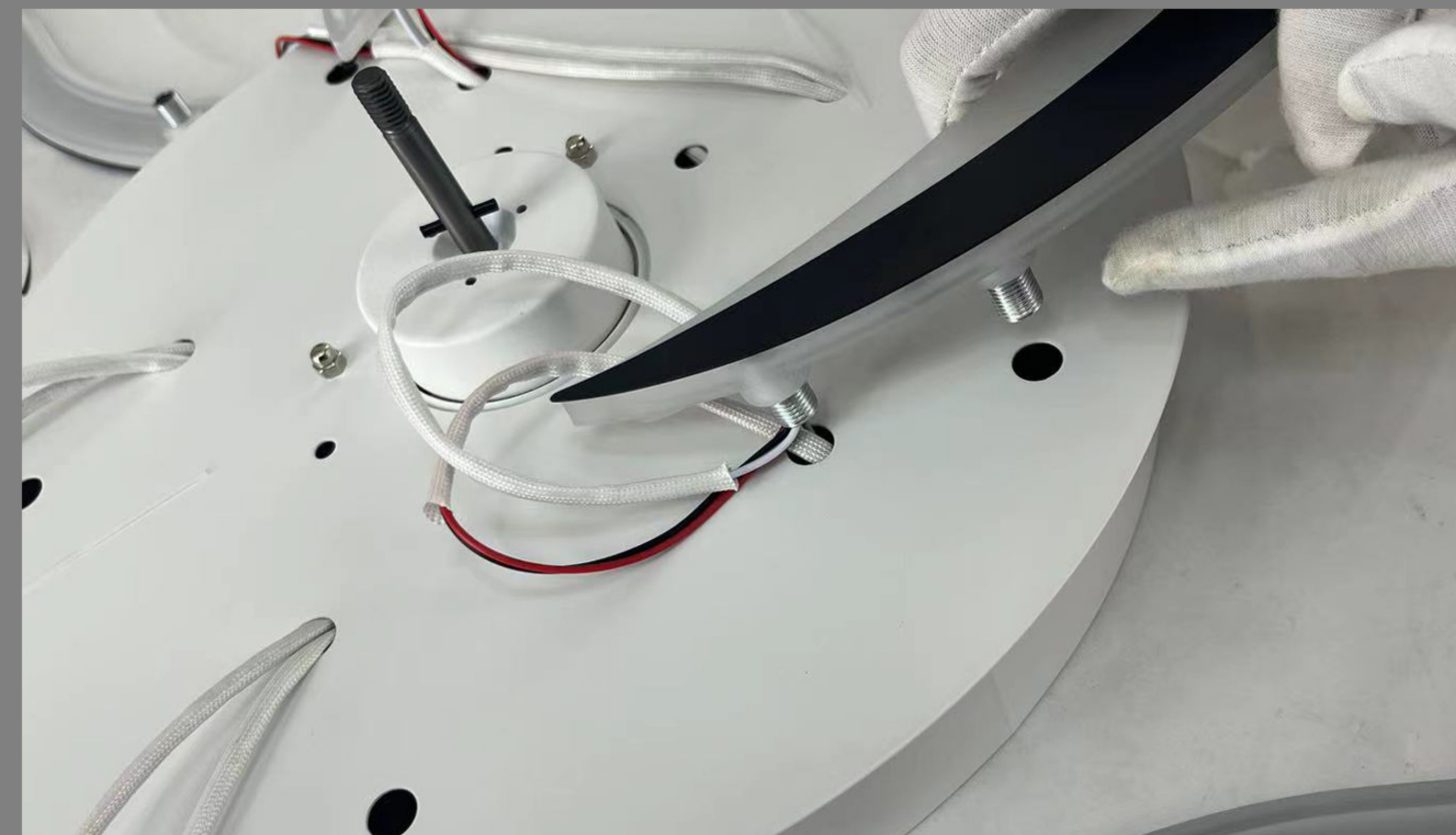
Step 2: Install all the petals, and fix them with nuts.
