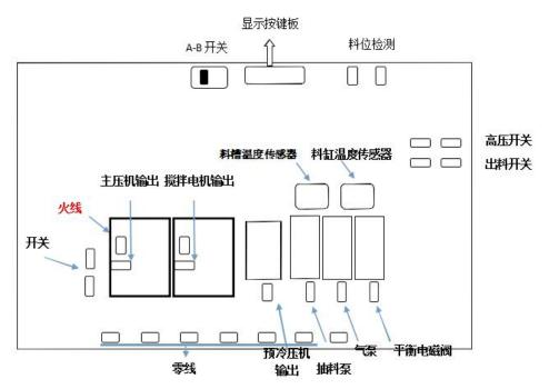
A-B 开关=A-B switch 料槽温度传感器=Material trough temperature sensor 料位检测=Level check 料缸温度传感器=Material cylinder temperature sensor 高压开关=High pressure switch 出料开关=Discharge switch 气泵=Air pump 主压机输出=Output of main press 搅拌电机输出=Output of mixer motor 火线=Fire wire 零线=Zero line 开关=switch 预冷压机=Precooling press 平衡电磁阀=Balanced solenoid valve 输出=output 抽料泵=transfer pump
