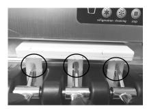
④ Install the handles to the valve stems one by one ,in the mean time, slowly push the steel pin through the discharger and the handles. (Refer to below photo for the correct direction of the handles)
