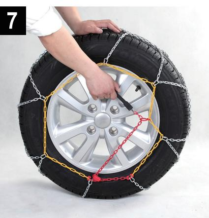
Pass the red chain into the red self-locking slide gear.
