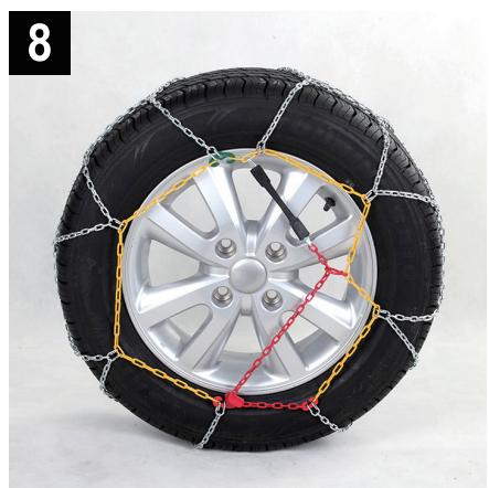
Thread the elastic tensioner into the red metal ring and then by pulling it as much as possible, fasten the elastic tensioner into a link of the side chain.
