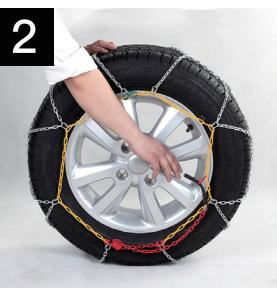
Unhook the elastic tensioner and release the tensioning chain first from the red ring, then from the red slide gear.
