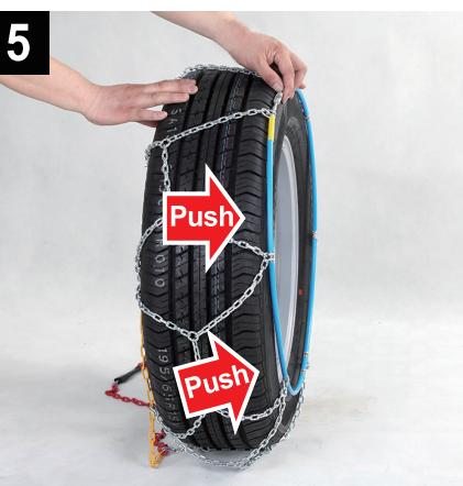
Push the flexible cable towards the interior of the wheel and make sure it is not on the tyre tread.
