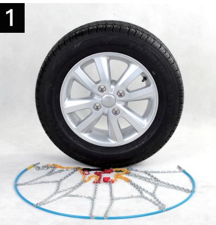
Unfold the chain on the ground, with the yellow plastic end of the cable towards the left.
