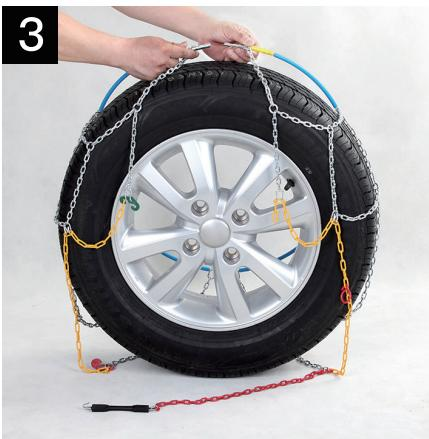
Pull upwards the flexible cable so that the two steel ends can be fastened together.
