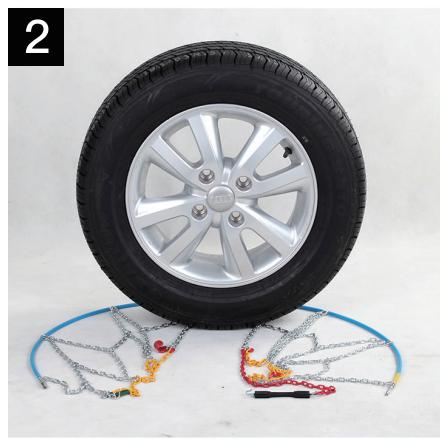
Pass the flexible cable (yellow plastic end first) behind the tyre from the left to the right.
