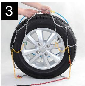
Unfasten the cable and allow the chain to fall down to the ground. Move the vehicle enough to release the chain from beneath the tire. (For front-wheel drive vehicles it is better to turn the wheels to make unfastening the inside cable easier).
