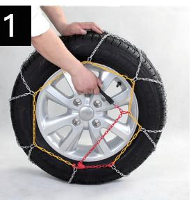
Stop the vehicle so that the outside flat green hook is in the upper of the wheel for vehicles with rear-wheel drive (towards the front for vehicles with front-wheel drive).
