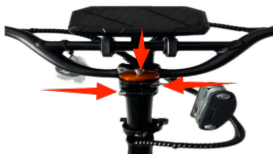
3. Adjust the angle and fasten it Screws
