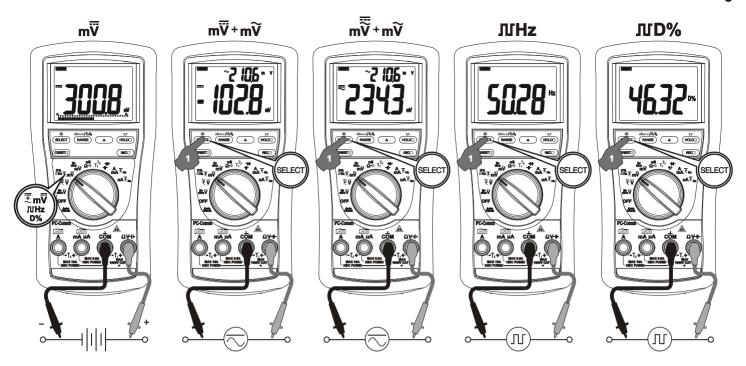
ACmV +Hz, dBm +Hz (Model 829s only), Hz +ACmV functions
