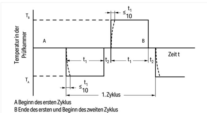
To simulate such conditions, the test specimen is exposed to repeated temperature changes, for example, between T<sub>A</sub> -40°C (-104°F) and T<sub>B</sub> +70°C (+158°F).
