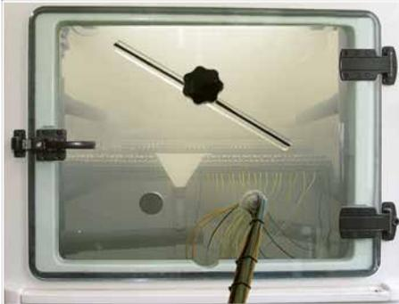
Depending on the test procedure being used, the test specimen is sprayed with salt mist for 16 hours up to 672 hours (4 weeks).
