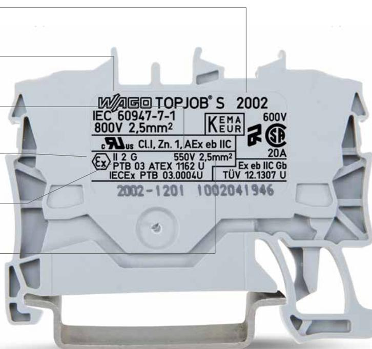
The embossed details on the terminal blocks show the manufacturer's name, the series number, the approval number, the approval data and the name of the testing authority. The type of protection Ex eb IIC Gb shown on the label or on the smallest packaging unit.
