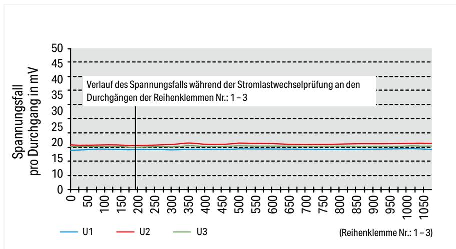
Voltage drop variation over longer periods under current load cycling conditions is shown for WAGO 285-195 (95 mm²/4/0 AWG) Rail-Mount Terminal Blocks using solid copper conductors. The diagram shows that the voltage drop is constant, far beyond the 192 cycles required in IEC 60947-7-1.
