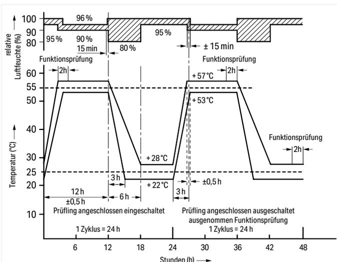
In addition to the salt spray tests, the damp heat test is also used for marine approvals.
