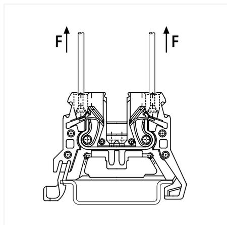
Test Arrangement per UL 486C:
