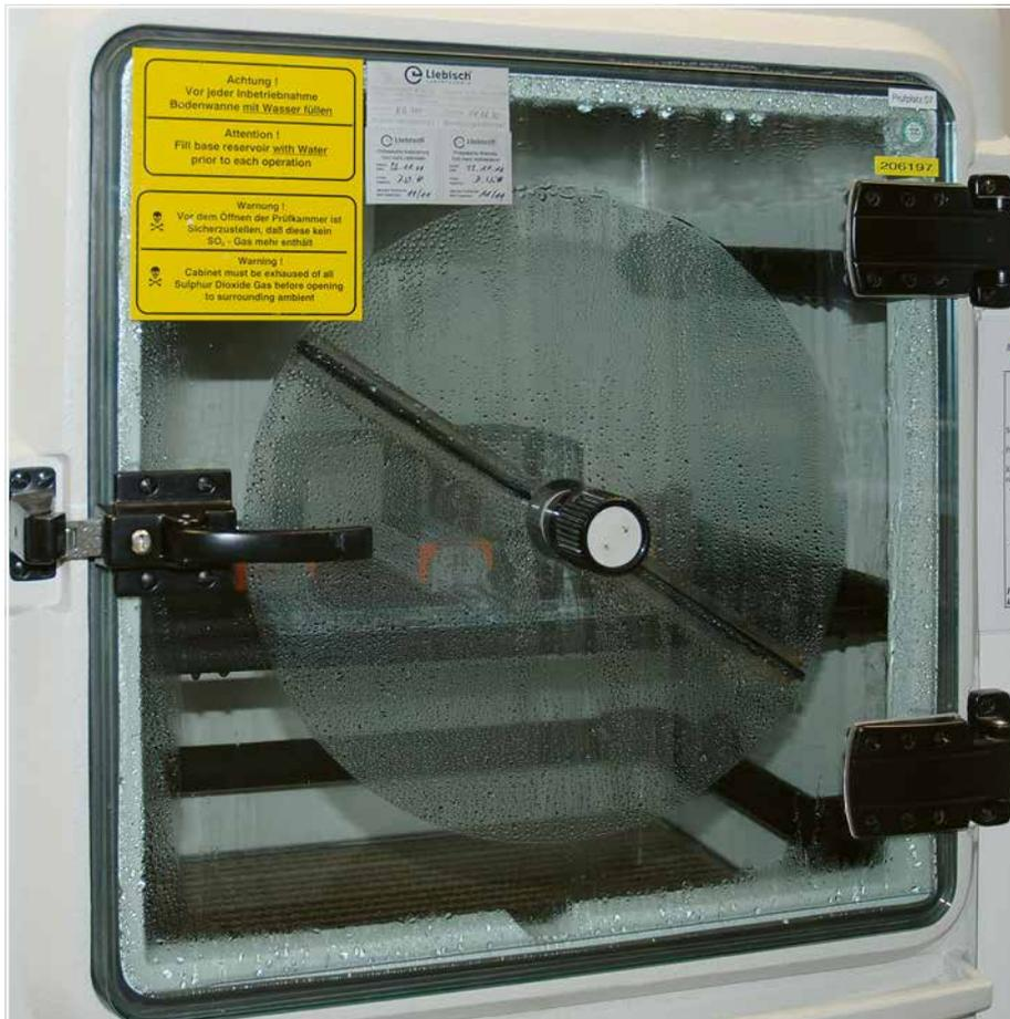
A saturated atmosphere is first created in a climatic chamber by heating an aqueous sulphur dioxide solution. After less than half an hour, the test specimen is fully saturated by the condensing vapors and exposed to this atmosphere for eight hours.
