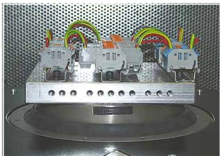
Other test types are performed using a single fixed frequency. The exact test procedure may vary considerably, depending on how the product will be used. Some test specifications require the determination of possible resonant frequencies, i.e., determining if resonance occurs within the frequency spectrum to be passed through. Analyzing the specimen behavior under the influence of resonant frequencies is performed using a special testing procedure.
