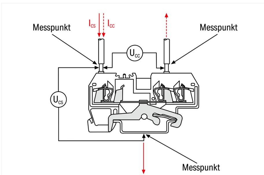
During the short-time withstand current test, the ground conductor rail-mount terminal blocks are subjected three times for one second each to a current load of  $120 \text{ A/mm}^2$ . The pass criterion for the test is the voltage drop (limiting value and constant measured values).
