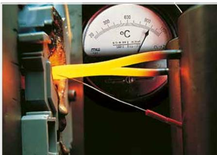
However, the glowing conductor shall not cause ignition of the product involved (e.g., a rail-mount terminal block). For the glow-wire test, the tip of the glow-wire is pressed against a surface of the test specimen (see picture).
