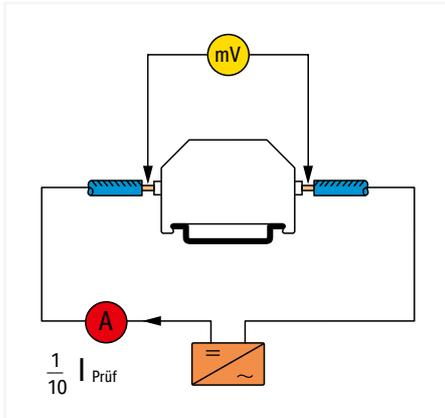
The CAGE CLAMP® and Push-in CAGE CLAMP® connections enclose and contain fine-stranded conductors. Therefore, a variation of the voltage drop with solid and fine-stranded conductors is so small that its influence may be negligible for the practical application of the terminal blocks.
