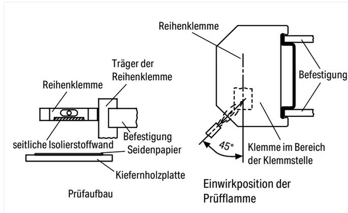
Flames must not be fuelled by the insulation materials used, thus creating a larger fire. The test specimen is exposed to a standard gas flame during a defined time period (e.g., ten seconds).
