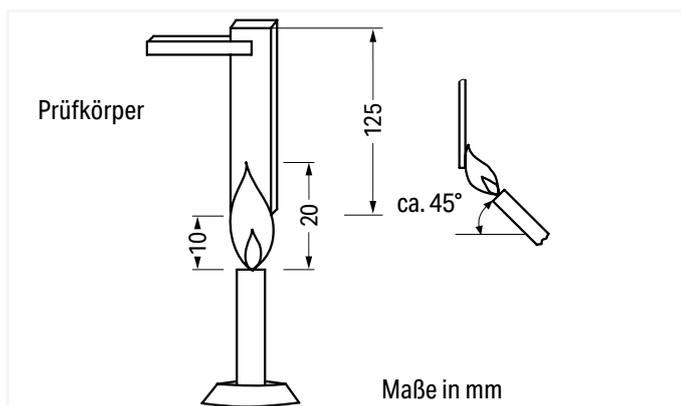
During the test, a 3/4 inch (20 ± 1 mm) flame is applied for two 10-second intervals to the specified bar specimen held vertically.
