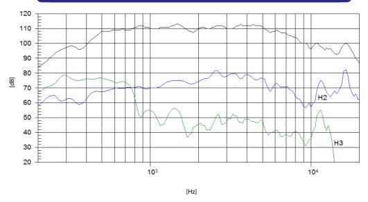
Note: On axis frequency response measured coupled to TD-460/N horn in anechoic chamber, 1W @ 1m
