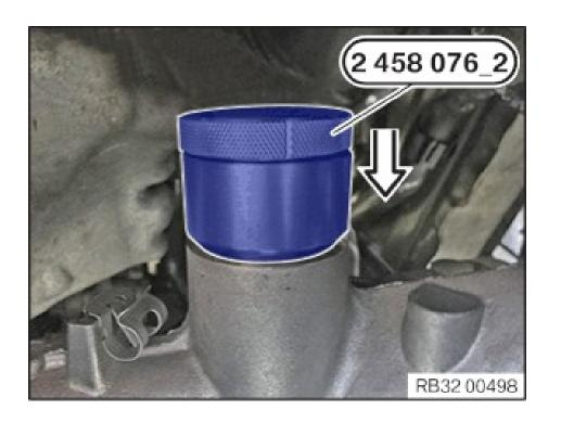
Press thrust piece with special tool 076\_22 458 (assembly tool) into the steering gear by hand.
