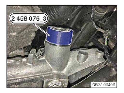
Screw special tool 076\_32 458 (sleeve) with thrust piece engaged into steering gear up to limit position.
