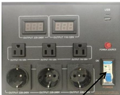
Power switch ( Air switch )
