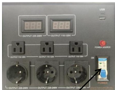
Power switch ( Air switch )
