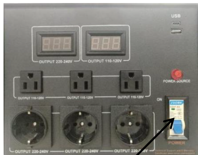
Power switch ( Air switch )
