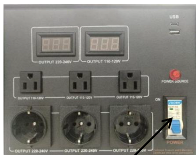
Power switch ( Air switch )
