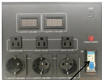
Power switch (Air switch)
