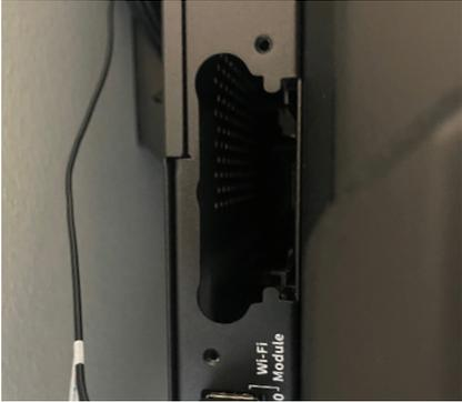
2. Insert the Wi-Fi Module into the port until firmly seated, then use the 2 screws to secure it.
