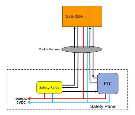
The above drawing shows the fundamentals of a sample system application. In factory automation, there are two main standards regarding functional safety requirements and implementation: (IEC) 61508 and (ISO) 13849. According to these standards, the safety relays used in the safety panel should comply with SIL3, PLD, or CAT4 categories.
