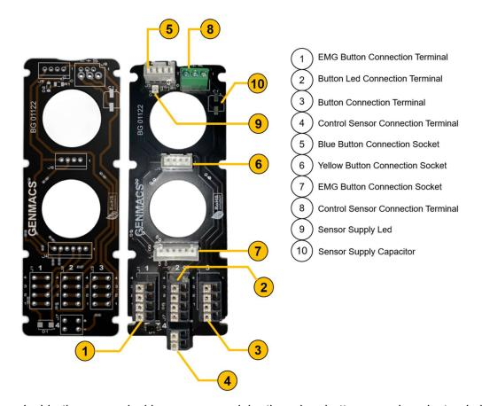
Inside the secure locking sensor module, there is a button grouping electronic board located at the bottom of the enclosure. This board is designed to provide connection convenience to the user by consolidating the connections of the existing 2 buttons and 1 emergency stop button on the enclosure, as well as the connections of the control sensor, at a single point. The circuit elements and connection points on the board are shown in the image above.
