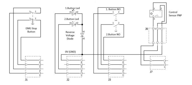
The pin assignment of the circuit grouping board is shown on the diagram above. In button group and inductive sensor-equipped product models (e.g., GSS-DLH-L-11), the connections are pre-wired for the sockets labelled J4, J5, and J6, as well as the terminal J8 on the board.
