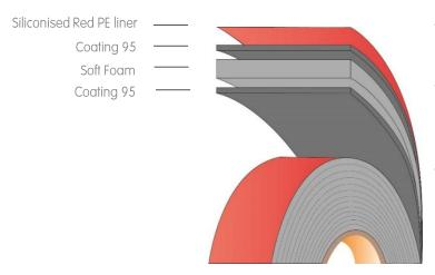
Thickness: 1,1 mm (0.047 inch) ± 10% High Conformable soft Core: foam acrylic
