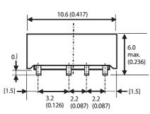
Tolerance of lead pitch is  $\pm 0.15$ mm (0.006inch) Other tolerances ±0.3mm (0.012inch)
