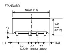
Tolerance of lead pitch is  $\pm 0.15$ mm (0.006inch) Other tolerances ±0.3mm (0.012inch)
