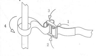
Installation steps six: fixed the bottom and rope
