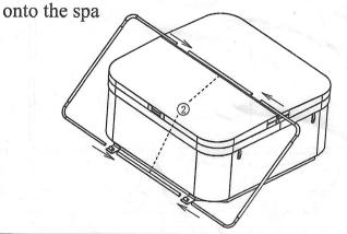
Installation steps Two: Install the stents on both sides respectively
