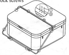
Installation steps seven: adjust the length of the rope
