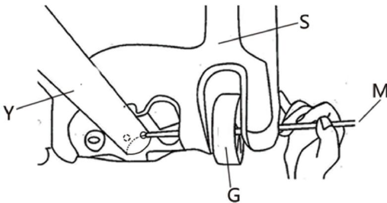
Insert the Wheel Shaft (M) into Wheel(G), Base(S) and end of Bottom Pole (Y) as shown.
