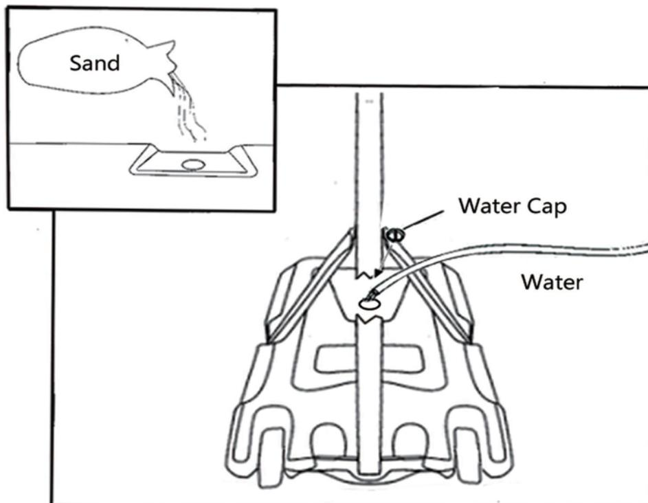
Filling the Base(S) with water or sand to keep steady.
