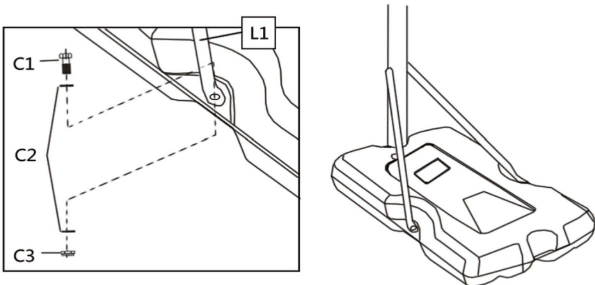
Fix the other end of Pole Brace(L1)&(L2) on two sides of Base(S) by Bolt Set (C1), (C2)&(C3) as shown.
