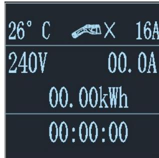
2.1 Adjust the charging current: click the button to adjust the charging gear. For EV-B07-EU022B,32A-24A-20A-16A-32A Cycle the current in this order. For EV-B07-EU011B,16A-13A-10A-8A-16A Cycle the current in this order. After switching the usage current, plug in the gun head to charge.
