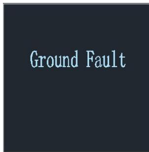
4.2 **Ground Fault:** The ground wire is not connected or the ground wire is poor. When this alarm message appears, please check if the grounding is normal. After ensuring reliable grounding, press the H button for 5
