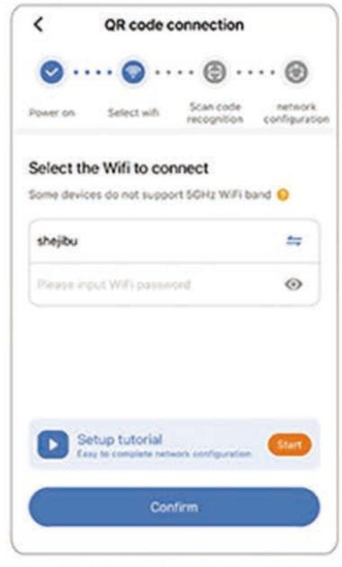
Note: The device only supports 2.4GHz Wi-Fi. Please select Wi-Fi without 5G". The name of Wi-Fi should not contain special symbols.
