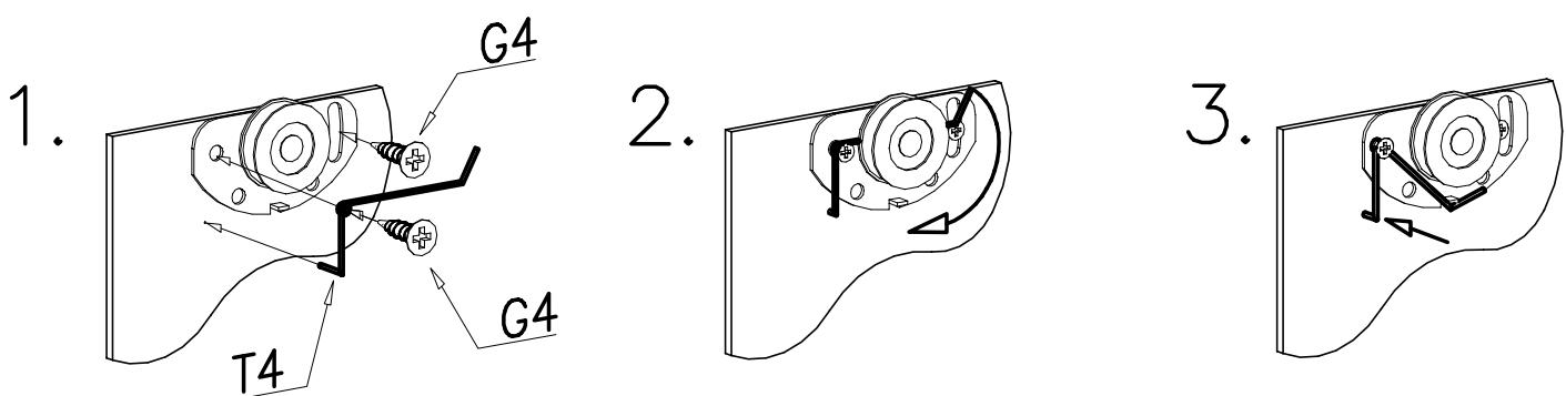
**GB** The G4 screw with the T4 element is screwed in so that there is a small clearance allowing the rollers to bend on the spring.
