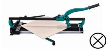
Put tile on the machine against the adjusted angle ruler.
