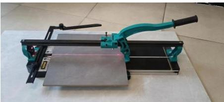
Place the cutting wheel on the rear edge of the tile
