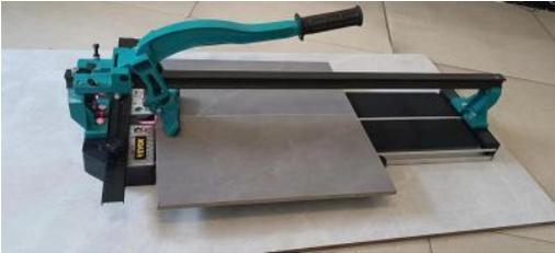
After scoring and without moving the tile position, the breaker is slightly in the front edge of the tile and front stop.
