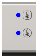
Fig. 12 Indicator light for chamber and boiler heaters
