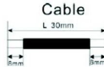
Insert striped cable into female terminal and crimp female terminal as shown below charts.
