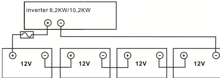
4. Insert the battery wires flatly into battery connectors of inverter and make sure the bolts are tightened with torque of 2 Nm in clockwise direction. Make sure polarity at both the battery and the inverter/charge is correctly connected and conductors are tightly screwed into the battery terminals.
