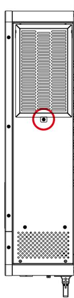
**Step 2:** Then, dustproof case can be removed and take out air filter foam as shown in below chart.
