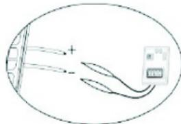
**CAUTION:** Exceeding the maximum input voltage can destroy the unit!! Check the system before wire connection.
