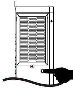
Once the unit has been properly installed and the batteries are connected well, simply press On/Off switch (located on the bottom of the case) to turn on the unit.
