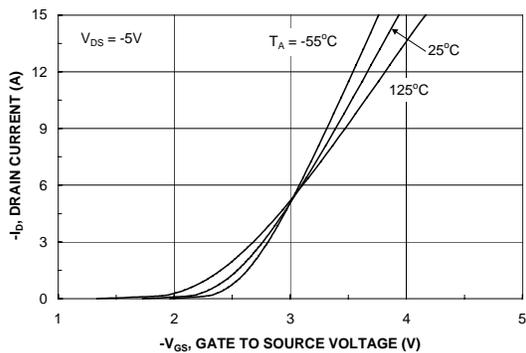
Figure 5. Transfer Characteristics.
