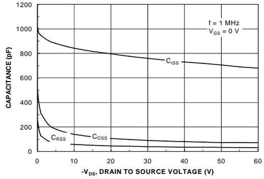
**Figure 8. Capacitance Characteristics.**
