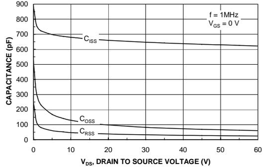
Figure 18. Capacitance Characteristics.
