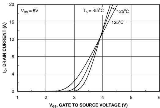
Figure 15. Transfer Characteristics.
