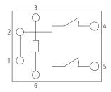
Pattern shall be designed to short-circuit #4 and #5 on the PC board.
