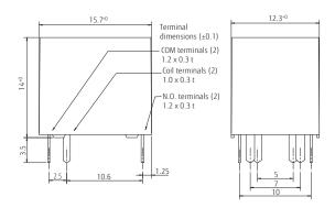
Dimensions of the terminals do not include thickness of pre-solder.
