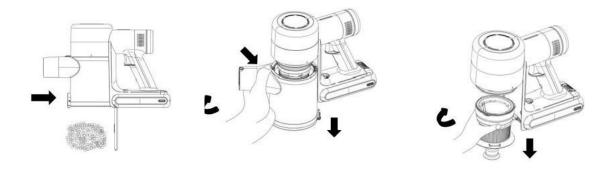
Turn off the host and press the release button to remove dirt.
