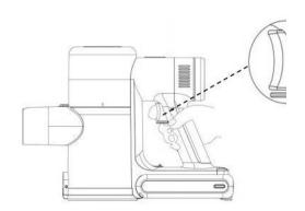
Press the switch button, the vacuum cleaner will immediately run
