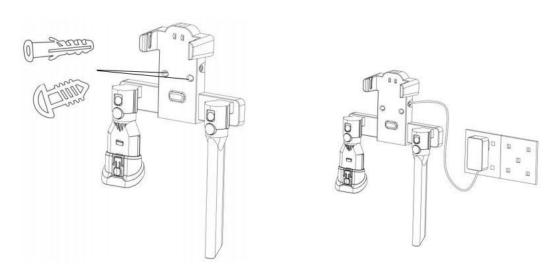
After fixing the wall hanging against the wall with screws, place the machine on the wall hanging and place the accessories in the left and right slots of the charging dock .
