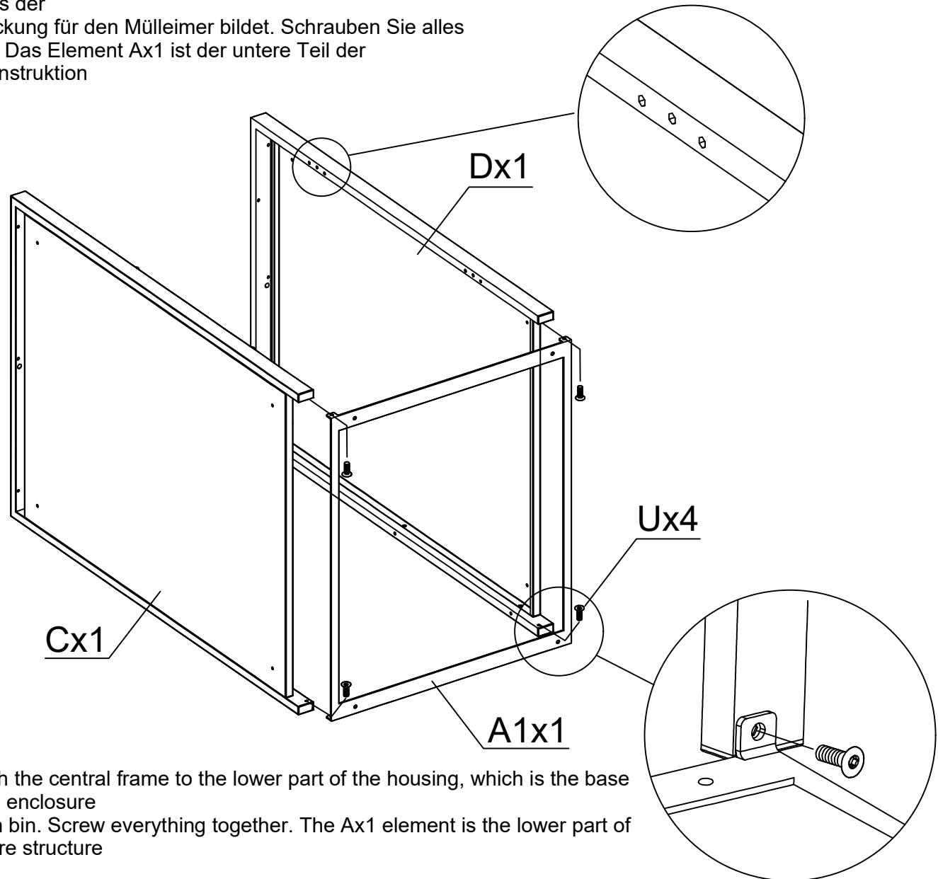
**ENG:** Attach the central frame to the lower part of the housing, which is the base of the metal enclosure for the trash bin. Screw everything together. The Ax1 element is the lower part of the enclosure structure
