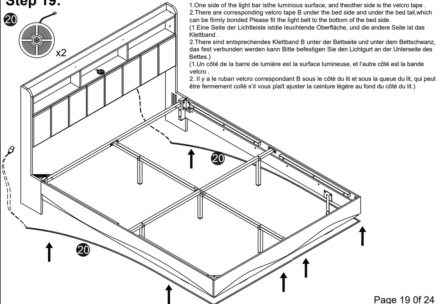
1. One side of the light bar is the luminous surface, and the other side is the velcro tape .
