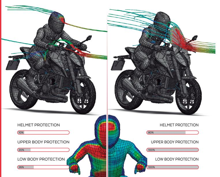
TOTAL DISSIPATED PRESSURE WITH PUIG SCREEN IS EQUIVALENT TO 6,5 Kg
