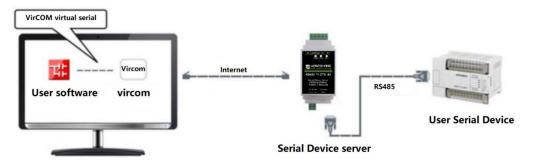
Figure 12 Application example of virtual serial port
