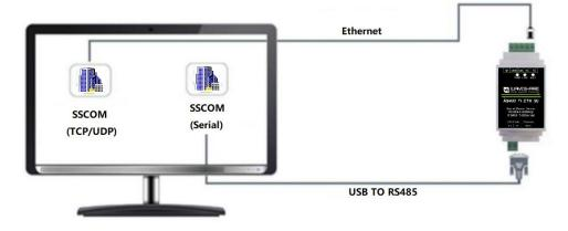
Figure 9 Schematic diagram of TCP communication
