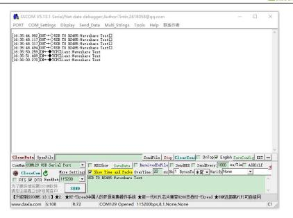
Figure 10 SSCOM1: USB TO RS485 transceiver interface
