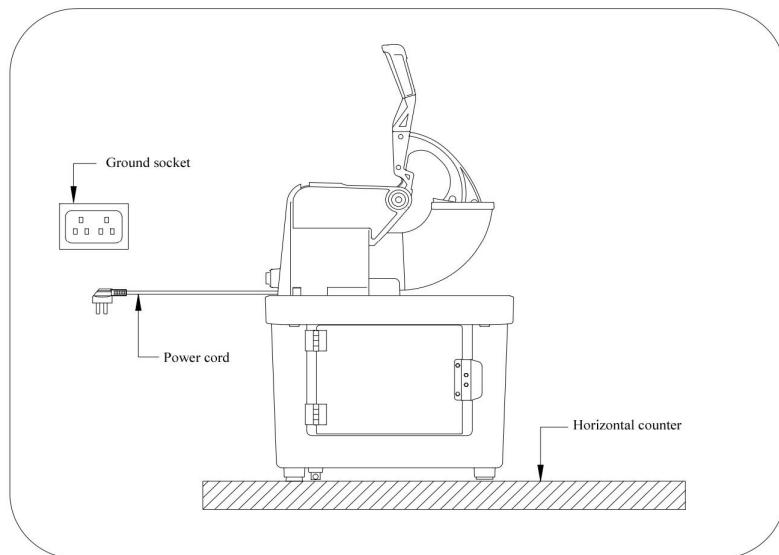
2. Find a flat location for the appliance where it's protected from direct sunlight and other heat sources (i.e., stove, furnace, radiator). Place the appliance on a level surface. Ensure at least 15cm of space between the back and sides of the appliance and the wall. Don't place anything on the appliance.
