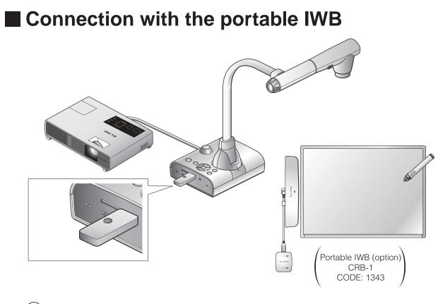
) Set up the device as shown in the figure above and connect to the projector, and then turn on the power.
