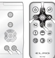
(2) You can display the selected picture/movie fullscreen by pressing the [  $(\square)$  ] button on the operating panel or the [ (AF) ] button on the remote control.
