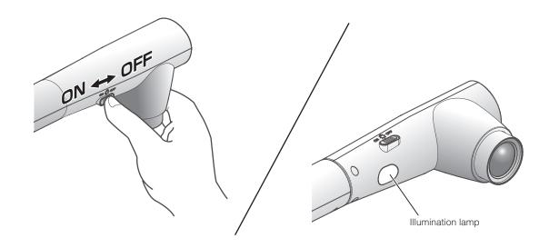
The illumination light can be turned ON/OFF by sliding the illumination light switch.
