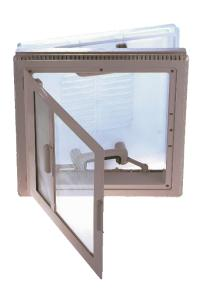
400 x 400 mm **Aperture** Roof thickness 24-56 bzw. 42-70 mm Corner radius 23 mm Site dome 470 x 470 mm Height over roof 91 mm Ventilation 150 / 30 cm<sup>2</sup> Weight 2.5 kg Size inner frame 470 x 470 x 14 mm Outer frame material Polypropylene Dome material Polypropylene Speed limit 130 km/h Authorization ECE R43 -019649
