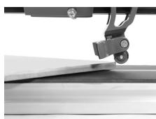
Place the cutting wheel on the rear edge of the tile.
