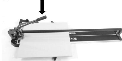
After scoring and without moving the tile position, the breaker is slightly in the front edge of the tile and front stop.
