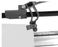
Make sure the breaker is upward to magnet on the sliding bar.
