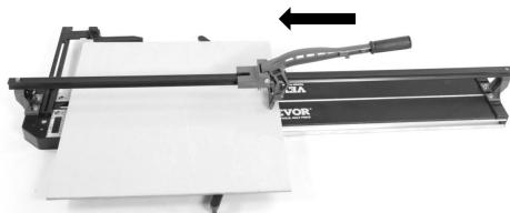
Place the cutting wheel on the rear edge of the tile.
