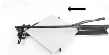
Put tile on the machine against the adjusted angle ruler.
