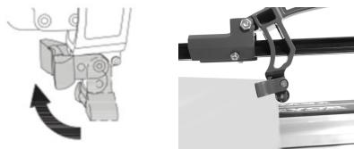
Slide the wheel forward by pushing the handle down with medium pressure.
