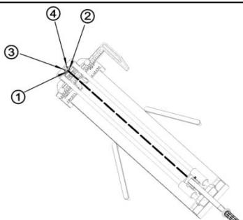
4, When the laser irradiation is too far/high, adjust the No. 3 and 4 screws clockwise.
