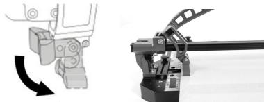
Raise the handle a little and release the breaker so that the breaker is flat on the tile.
