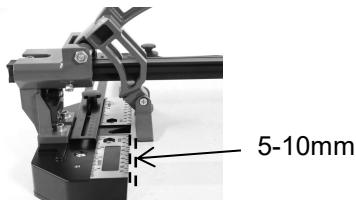
Tips: After scoring, it is better to pull back the handle to let the breaker slightly backtrack 5-10mm, it's the best position to break the tile.
