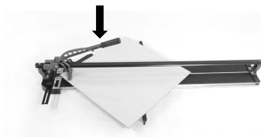
After scoring and without moving the tile position, the breaker is slightly in the front edge of the tile and front stop.
