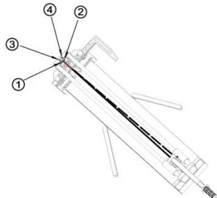
2, If the laser is biased to the left, adjust the No. 2 screw clockwise or the No. 1 screw counterclockwise.
