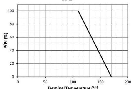
Full power dissipation is achievable with the part mounted on 120x51mm high-Tg FR4 board with 70µm inner and outer planes. Alternative mounting arrangements may be used, provided the heatsinking effect permits a combination of power dissipation and terminal temperature within the derating curve shown.
